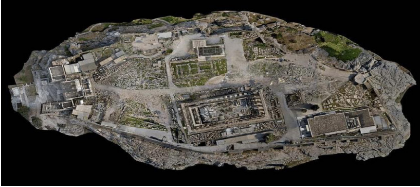
Figure 33. Acropolis laser scanning and photogrammetry orthographic results
